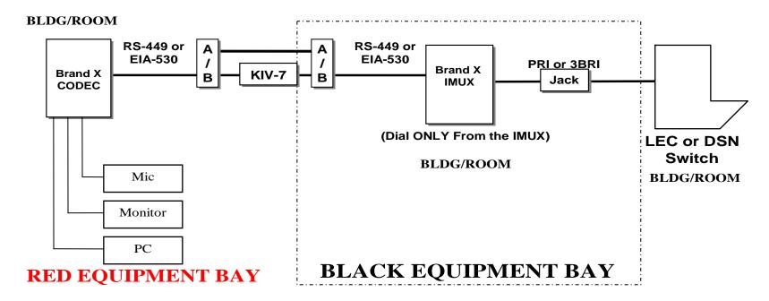
NOTE: This Configuration is only authorized with proper isolation integrated within the A/B Switch, such as optical isolation. (See the current list on the Approved Equipment page.)
