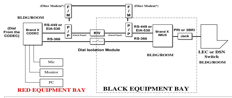
(Patch KIV-7 into path for Classified -/- Remove/replace with UNCLASS patch for Unclassified.)
