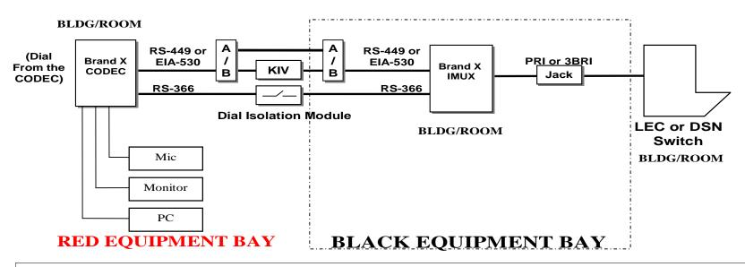
This Configuration is only authorized with proper isolation integrated within the A/B Switch, such as optical isolation. (See the current list on the Approved Equipment page.)
