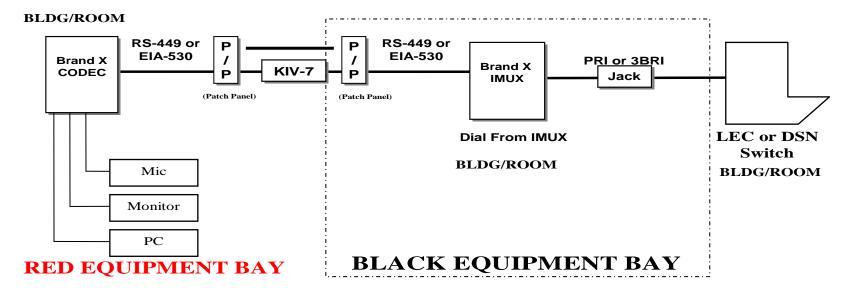
(Patch KIV-7 into path for Classified – remove/replace with UNCLASS patch for Unclassified.)
