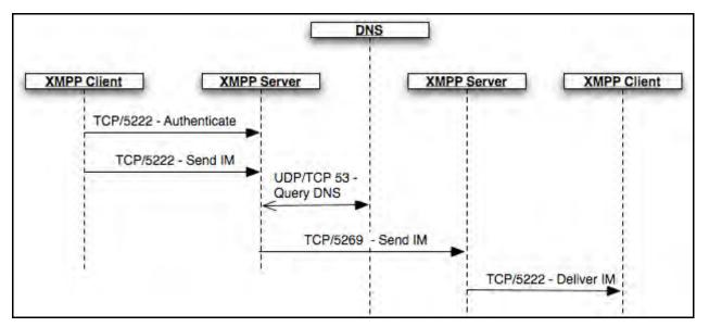
Figure 5.7.5.2-2. Routing of XMPP Messages
